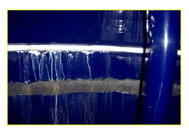
Pic.4 冷热温差急变引起的搪玻璃失效 Glass failure due to thermal shock/cold shock
