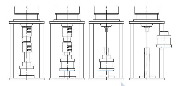
机械密封快速更换 Quick Change for Mechanical Seal
